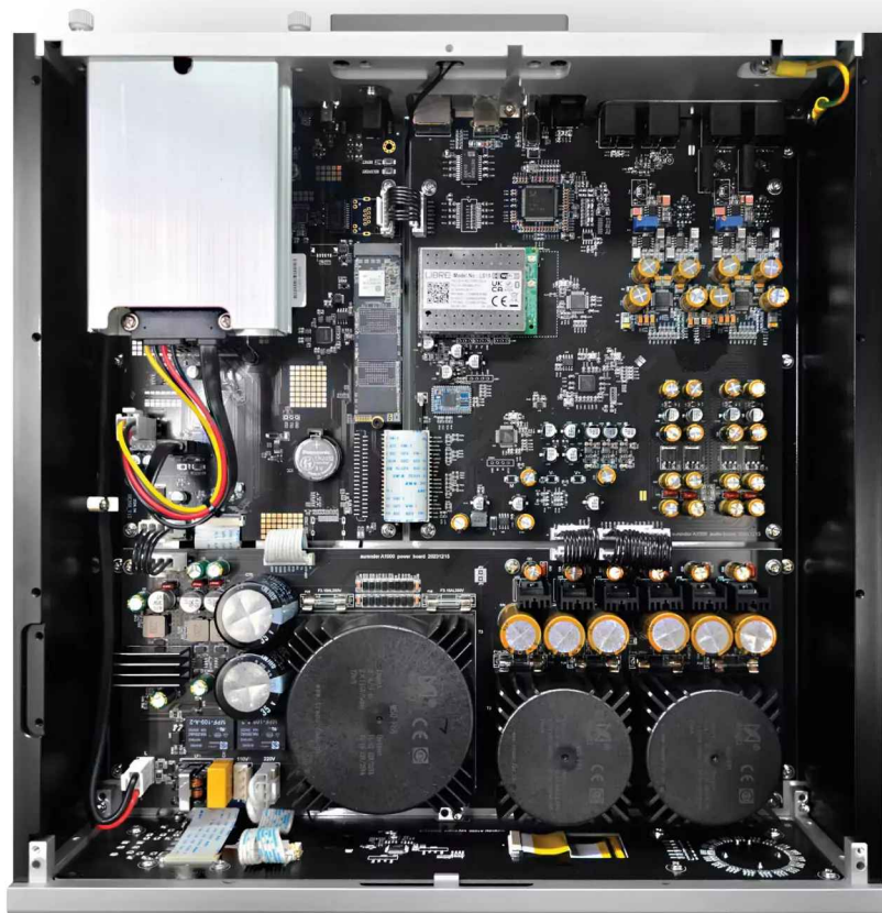
△ SEPARATE TRANSFORMERS ARE DEDICATED TO EACH OF THE ANALOGUE, DIGITAL AND DISPLAY/CONTROL CIRCUITS. DUAL AKM4490REQ DACS ARE NESTLED AMONG FOUR-CAPACITOR GROUPS UPPER RIGHT.
